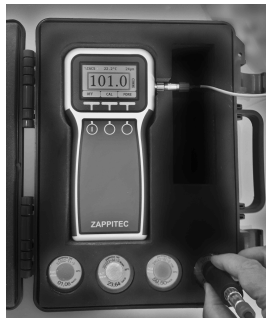
Figure 1: Meter model 1201 showing case and standard blocks
