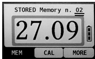
Figure 9: Meter Screen - Storing Value
