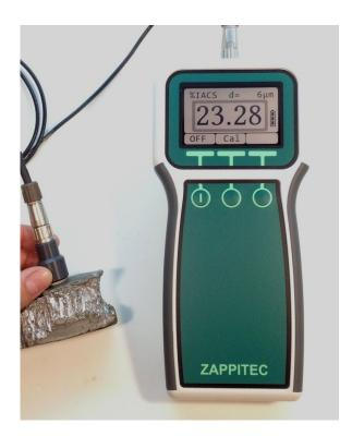
Zappitec is introducing the model **12Z** Eddy Current Electrical Conductivity Meter for non-magnetic metals. The **12Z** uses the latest technology to provide an instrument which is user-friendly and practical to measure electrical conductivity in the field.
